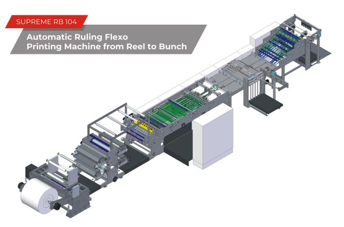
TRUTECH Automatic Ruling Flexo Printing Machine from Reel to Bunch with Cover consists of shaft-based reel unwinding stand, ruling / flexo printing tower, cross cutting unit, sheet overlapping unit, sheet counting and collating unit, inserter for pre-printed index sheets and title covers, pile delivery station and centralized control panel (PLC) with lubrication system.
