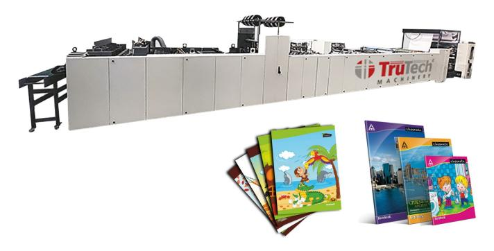
High Speed Automatic School Book Machine consists of shaft less reel unwinding stand, ruling / flexo printing tower, cross cutting unit, sheet overlapping unit, sheet counting and collating unit, inserter for pre-printed covers, pinning unit, folding unit, back pressing unit, front cutting, book partition unit and delivery table along with centralized control panel (PLC) with lubrication system. Connectivity for online support.
