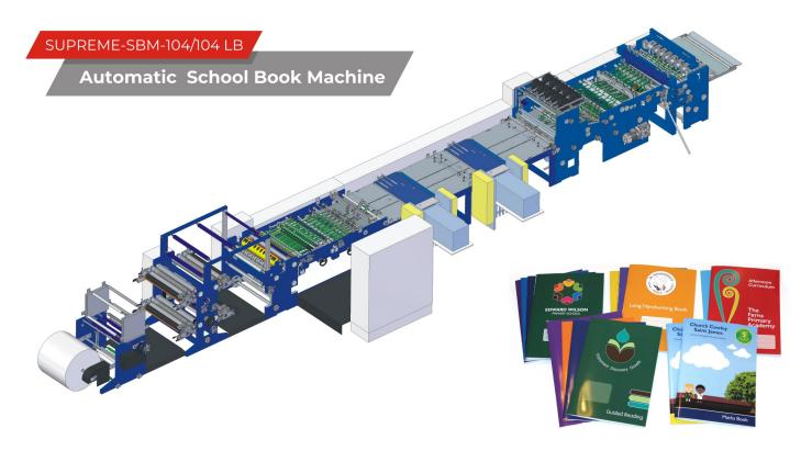
TRUTECH Automatic School Book Machine consists of shaft based reel unwinding stand, ruling / flexo printing tower, cross cutting unit, sheet overlapping unit, sheet counting and collating unit, inserter for pre-printed title/index sheet, pinning unit, folding unit, back pressing unit, front cutting, book partition unit and delivery table along with centralized control panel (PLC) with lubrication system.
