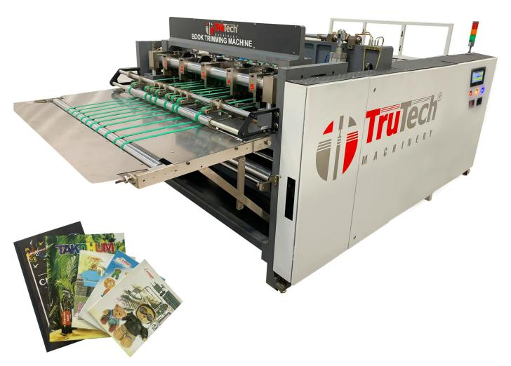
Book Triming Machine consist of automatic bunch feeding table, book front cutting unit, book partition cutting unit, book delivery table, waste removal trolley, lubrication system and centralized control panel (PLC).
