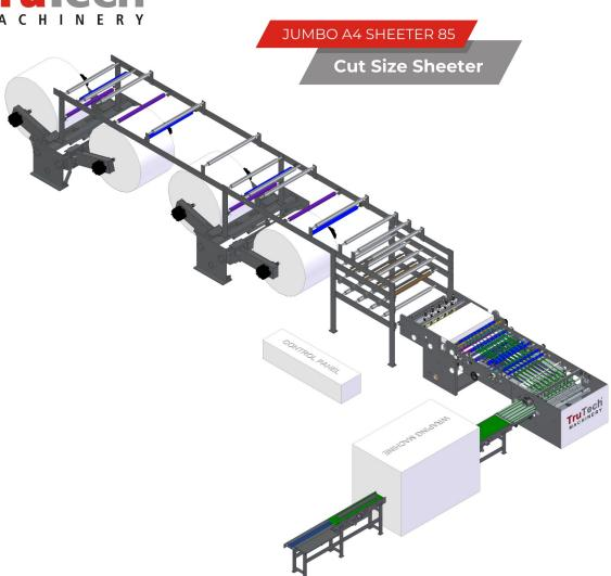
Jumbo A4 Cut Size Sheeter consists of shaft based unwinding one double reel stand, de-curling unit, slitting unit, rotary cutting unit, conveying unit, counting and collecting unit, ream wrapping unit and centralized control panel.
