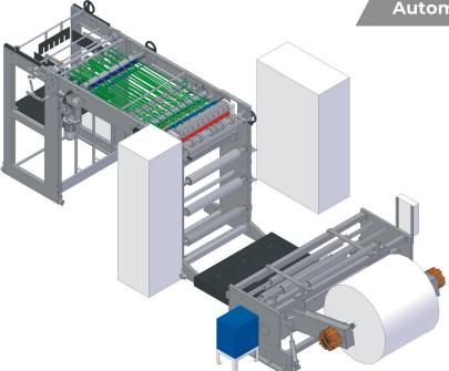
Automatic Folio Size Sheeter comes with latest technology for converting reels to sheets. The machine consists of shaft less reel unwinding unit, cutting tower, overlapping unit, pile delivery unit and air-conditioned two door pane.
